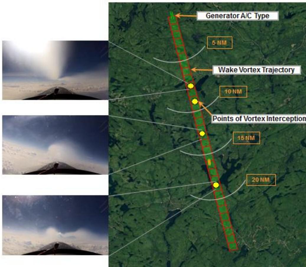
**Figure 1: In-Trail Wake Vortex Trajectory**
