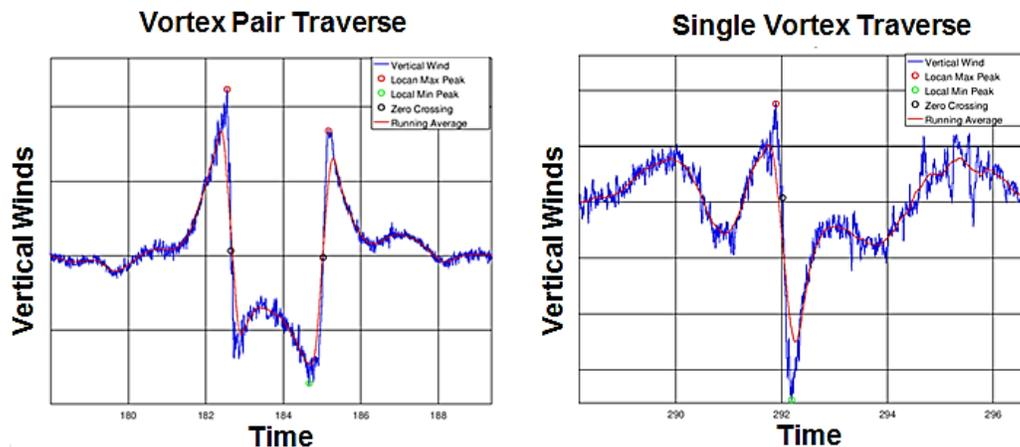
**Figure 3: Vertical Wind Component Plots**
