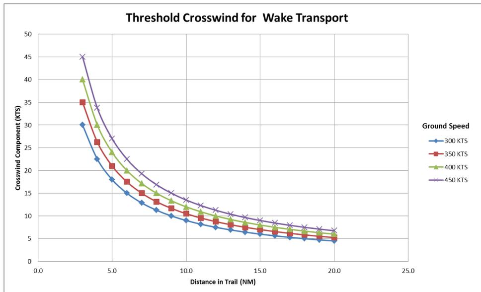
**Figure 4: Threshold Crosswind Analysis**
