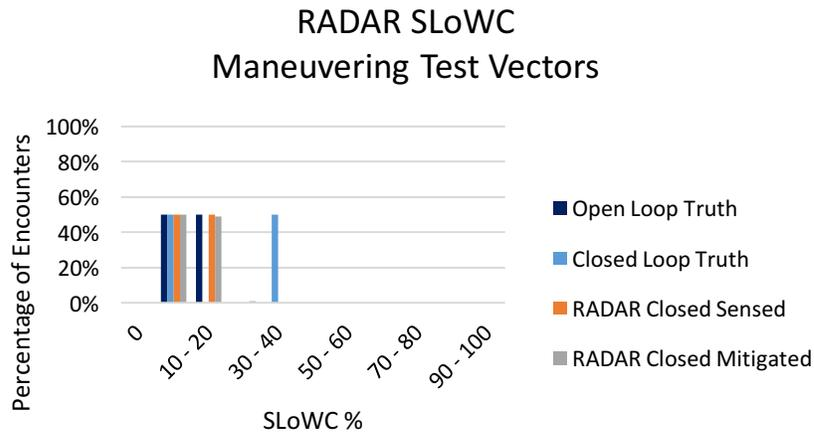
Figure 5. Radar SLoWC for Maneuvering MOPS Requirement-Derived Test Vectors
