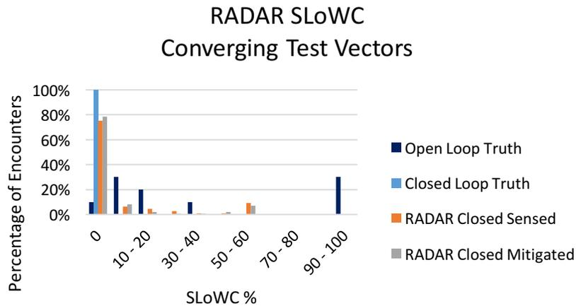
Figure 4. Radar SLoWC for Converging MOPS Requirement-Derived Test Vectors
